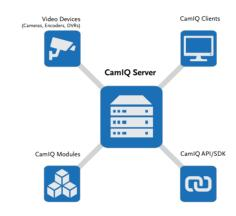
CamIQ 8 Satellite reliably analyzes, records and transmits video data. Prevalent types of network cameras and appropriate video servers can be used as image sources.
